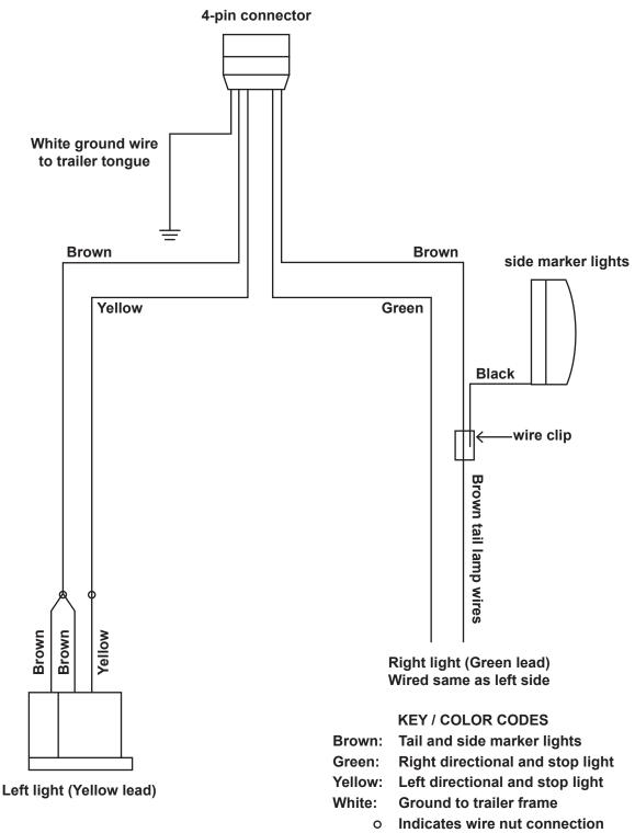
Figure K: Wiring Diagram
